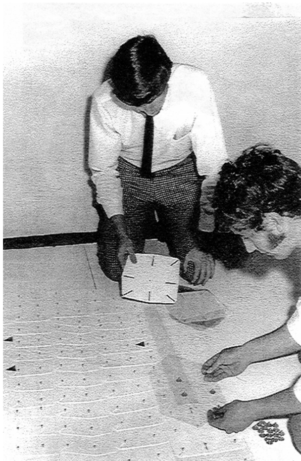
Fig. 12. Laying white 'Flovic' plastic templates and clear 'Cobex' plastic azimuth templates.
